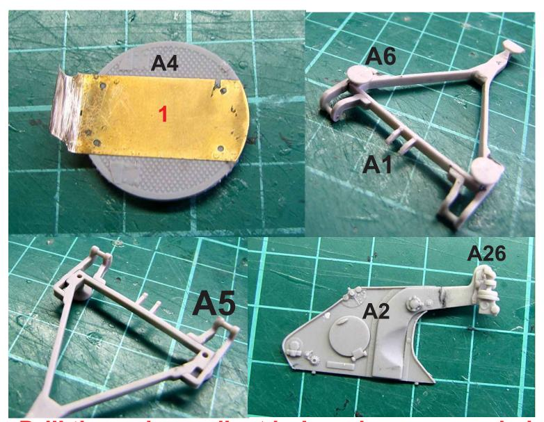
Drill through or adjust holes wherever needed
