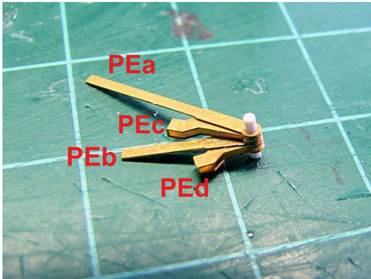
Levers and PE rings assembled on 0,8mm wire or rod 2,7mm long, resin handles added and whole thing mounted in place. Once again some other details added
